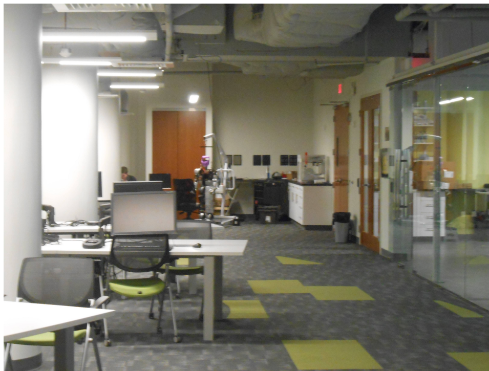
Figure 4.1: Photograph of the ExCITe Research Center workshop room. Noise sources include lights in the ceiling, ventilation ducts, and electronic locks on the doors which make a clicking sound when unlocking.
