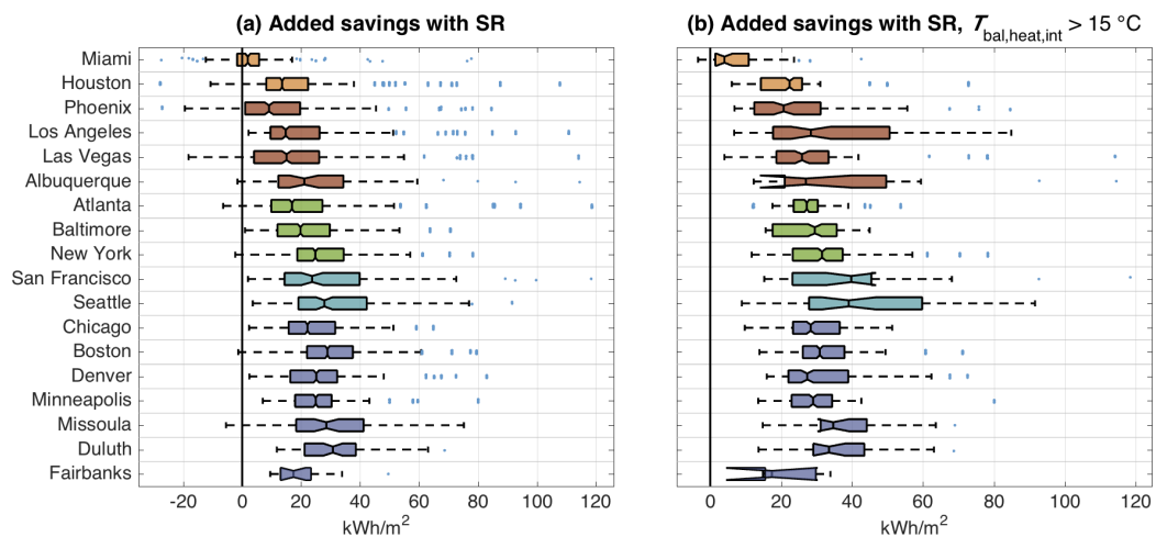
Figure 9 The HVAC source energy savings difference between Econ+SR and Econ in the medium-VAV office for (a) all instances and (b) instances where the heating balance point temperature (based only internal gains) exceeded 15 °C.
