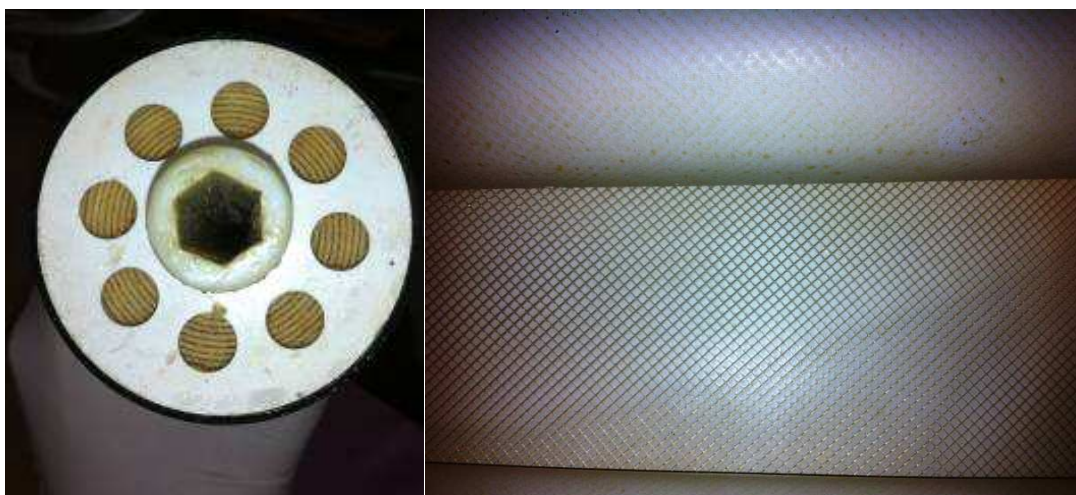
Figure 23 Pilot RO membrane after operation. The spiral wound membrane element opened during autopsy had evidence of biological fouling (source: the author).
