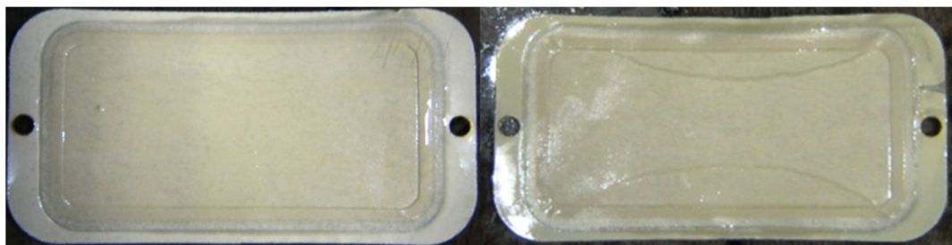
Figure 28 RO membrane from the membrane test cell (left: baseline feed test; right: acetate amended feed; source: the author).
