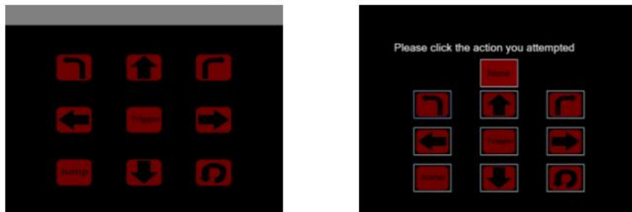
Figure 39: Left – the 3x3 P300 BCI matrix used. Right – the training manual selection screen. From [118].
