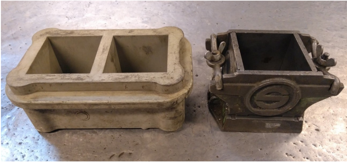
Figure 5.4. The moulds used for casting the 100 mm cube specimens for the compressive testing.
