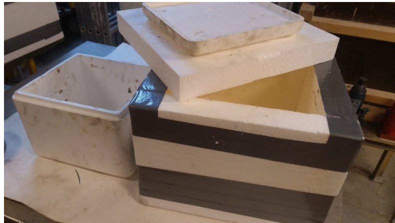
Figure 5.3. Picture of the isolating mould used for monitoring the temperature development of the different concrete classes. On the right, the additional insulation into which the original polystyrene box, left, was placed.
