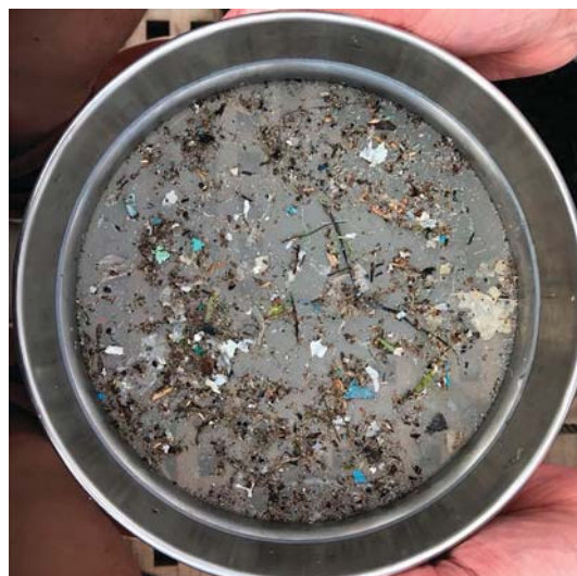
Figure 2. Plastic sample taken from an expedition in the Ligurian Sea in May 2018 by the “Sail and Explore Association” using a manta trawl during 30 min with a mesh size of 0.3 mm. The Mediterranean Sea represents one of the most polluted seas worldwide with nearly four times higher concentrations of microplastic fragments compared to the North Pacific Gyre and a record-breaking number of 1.25 million microplastic fragments per square kilometer floating. 53 Reprinted with permission from Sail and Explore Association, Copyright 2018.
