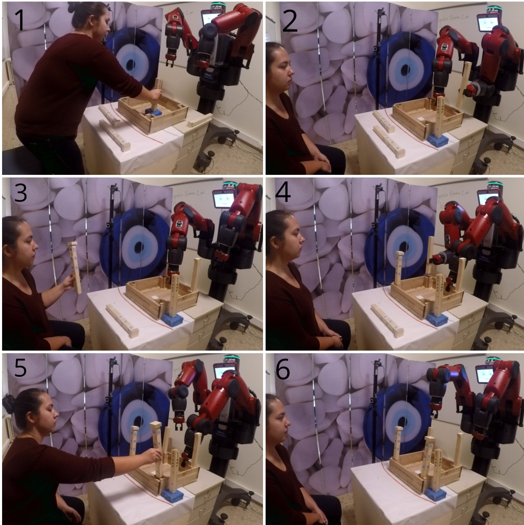
Figure 9: Physical experiment: In snapshot (1) the robot explained human that the stamp is too close to you, it will be safer if she can stamp the table; (2) the robot continues with the next assembly task; (3) the robot senses that human is holding a leg and confirms whether she wants to assemble it; (4) after the human assembled, robot assembles another leg; (5) robot asked human help to assemble a leg as it is not feasible for the robot to reach the leg (6) the robot picks foot with the sharp nail (dangerous task for human) to assemble it to the leg
