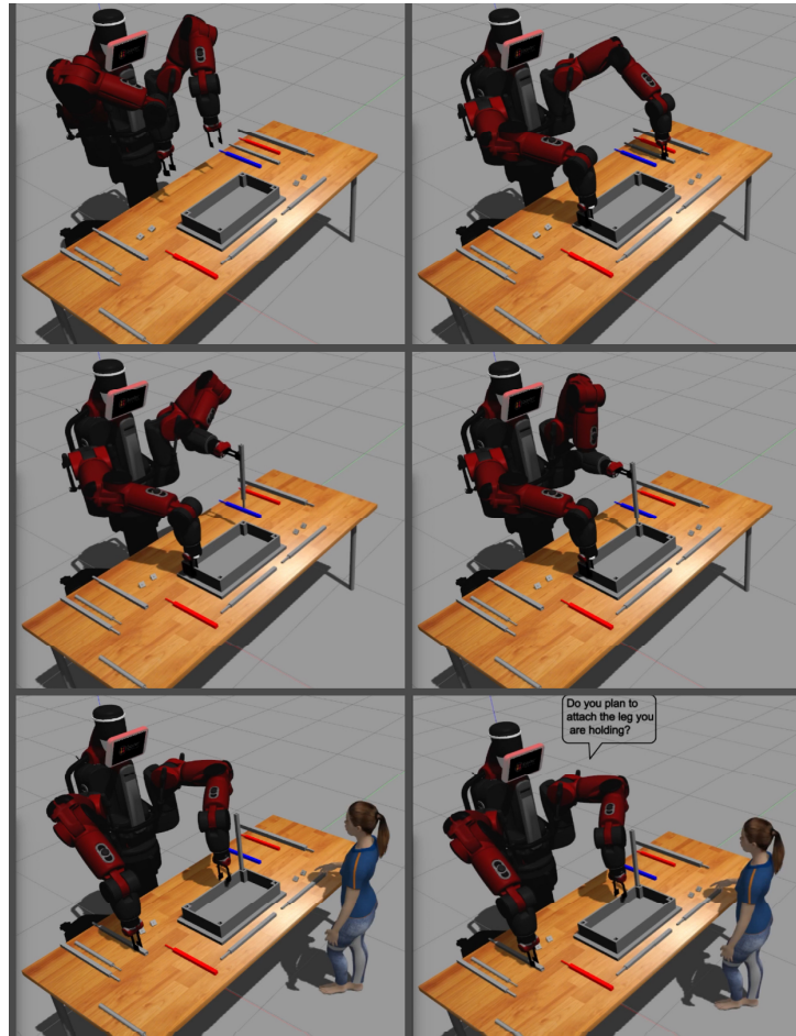
Figure 6: Simulation snapshots: Part 1. The robot assembles one of the legs to the table top. Then he notices that the human is holding a table leg, which can be assembled to the table top. The robot confirms with the human as to whether she is planning to attach the leg to the table top.
