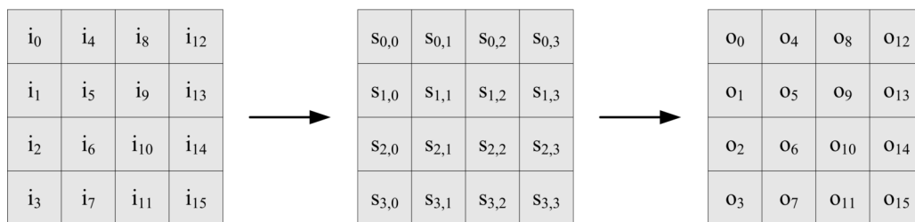
Figure 3.5: AES input, state and output transition
