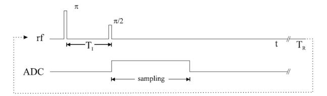
Figure 2.12: The sequence diagram for an inversion recovery experiment. ADC stands for analog-to-digital converter and converts the analog MRI signal to digital. Figure reproduced from [2] with permission.
