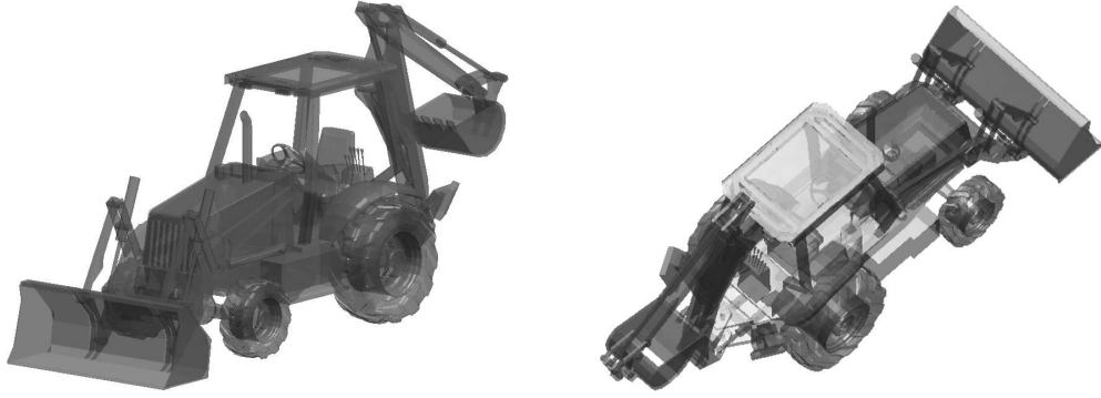
Figure 3.14: Backhoe model used in Xpatch scattering predictions. The view to the right corresponds approximately to the images in our experiments.
