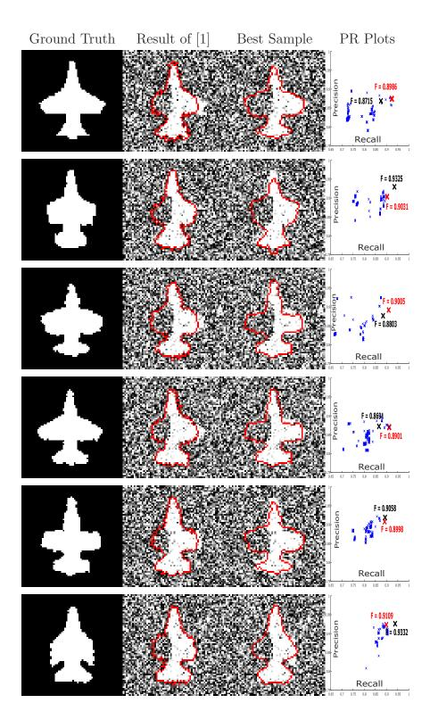
Figure 4.6: Experiments on test image set - 2 of the aircraft data set. Note that each row contains the results for a different test image. In the PR plots, ' $\times$ 'and ' $\times$ 'mark the samples produced by our approach where ' $\times$ 'indicates the sample with the best F-measure value, and ' $\times$ 'marks that of segmentation of Kim et al. [1].
