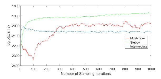
Figure 4.28: Log posterior probabilities of the samples obtained by running the algorithm on the test images in Figure 4.26.
