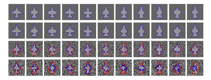
Figure 4.16: Marginal confidence bounds obtained from samples for each test image in the experiments with the aircraft data set. Note that red indicates the least confidence boundary whereas blue indicate the most confidence boundary.
