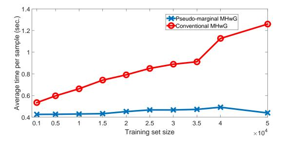
Figure 4.19: Average running time for producing a single sample as a function of training set size for both pseudo-marginal MHwG shape sampling and conventional MHwG shape sampling.
