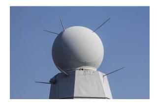
Figure 7: Active phased array example: SAMPSON[4]
