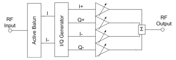
Figure 20: Block diagram of a typical vector sum type phase shifter
