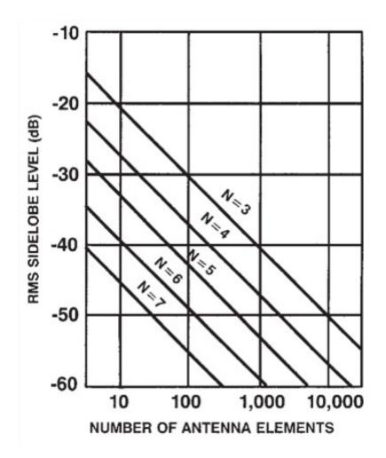
Figure 21: Required antenna number to reach the same RMS side-lobe level with different phase resolutions [6]
