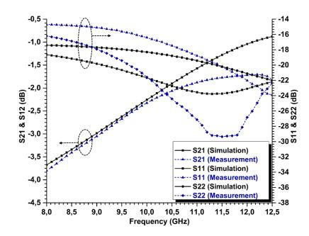
Figure 58: Simulation and measurement results of designed a new compact type gain-equalizer
