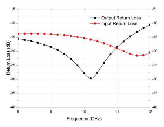
Figure 31: Simulation result of the return losses of the SP4T
