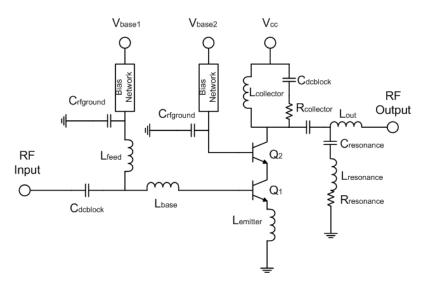
Figure 63: Schematic of an active gain-equalizer
