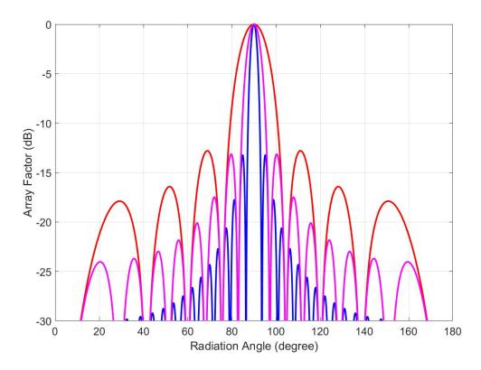
Figure 3: Normalized array pattern of a linear array with  $\lambda/2$  spacing for (red) N=8 (magenta) N=16 (blue) N=32 antenna elements
