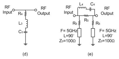
Figure 50: Examples of the schematic of passive gain-equalizers
