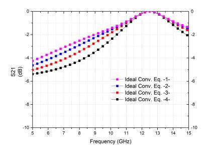
Figure 52: The gain vs. frequency for four example conventional gain-equalizers
