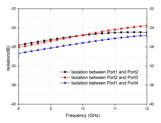
Figure 33: Simulation result of the isolation of the DP4T
