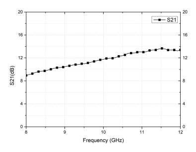
Figure 69: S21 measurement result of RX chain of T/R Module
