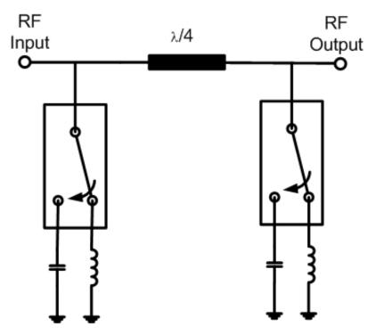
Figure 16: General diagram of the bit of the loaded-line phase shifter
