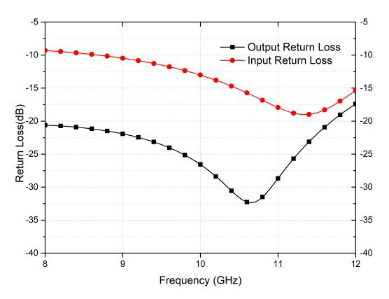
Figure 35: Simulation result of the return losses of the DP4T
