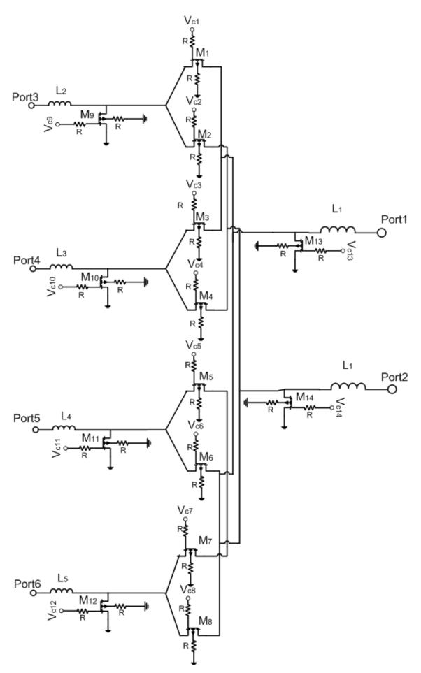
Figure 32: Schematic of the DP4T 44
