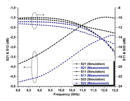
Figure 55: Simulation and measurement results of designed conventional type gain-equalizer
