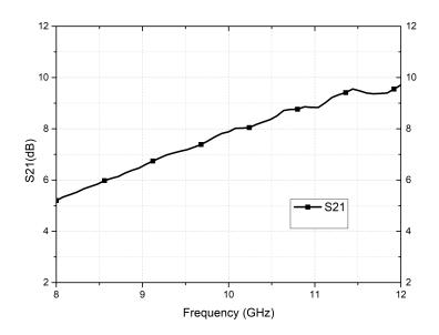
Figure 65: S21 measurement results of designed first active gain-equalizer
