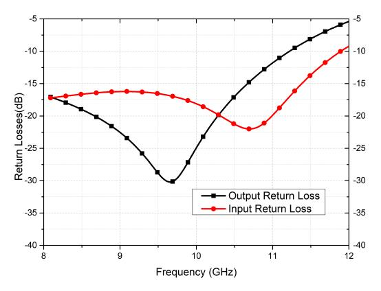
Figure 39: Simulation result of the return losses of the 4P4T
