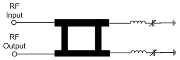
Figure 17: General diagram of the bit of the reflection-type phase shifter
