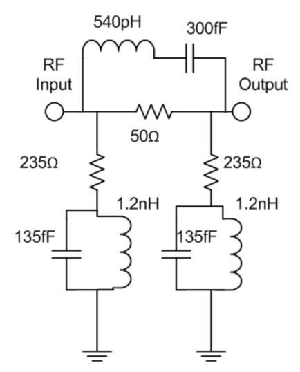
Figure 56: The schematic of designed a new compact type gain-equalizer
