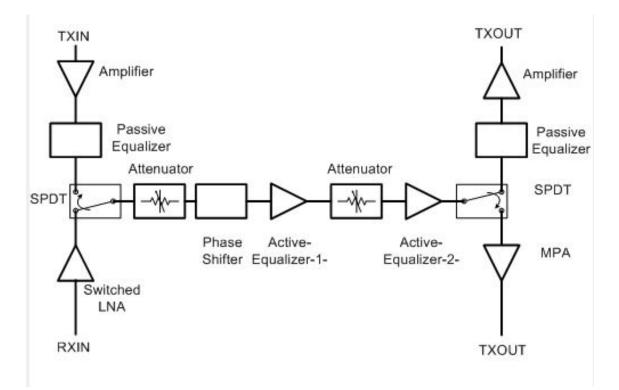
Figure 14: SiGe X-band all-RF T/R module block diagram and component specifications
