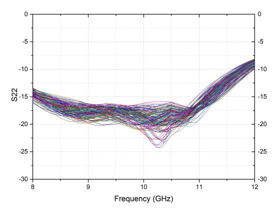
Figure 41: Simulation result of the output return losses of all states of the designed phase shifter
