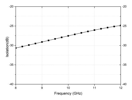
Figure 29: Simulation result of the isolation of the SP4T
