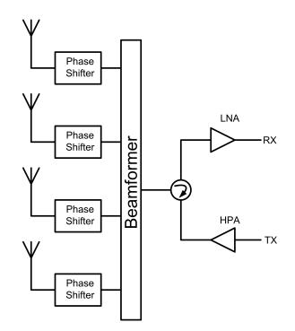
Figure 4: Block diagram of passive phased array
