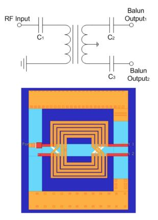
Figure 25: Schematic and Layout of the Transformer
