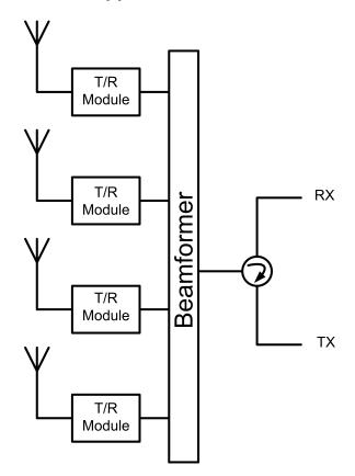
Figure 6: Block diagram of active phased array
