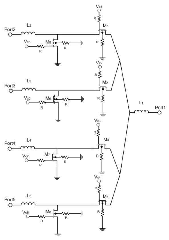
Figure 28: Schematic of the SP4T
