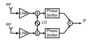
Figure 9: IF phase shifting Phased array architectures
