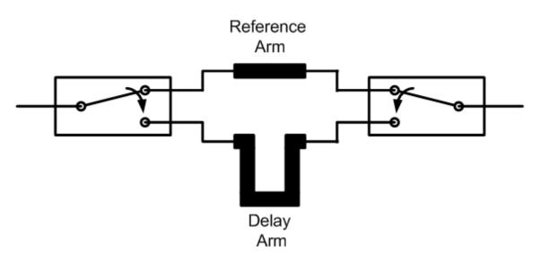
Figure 15: General diagram of the bit of the switched-line phase shifter
