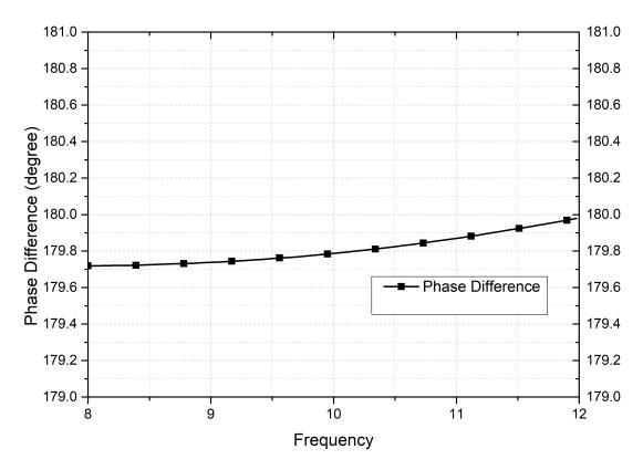
Figure 27: Simulation result of the phase difference between each output of the transformer
