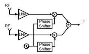
Figure 10: LO phase shifting Phased array architectures
