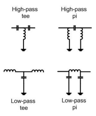
Figure 19: Tee and pi filter networks
