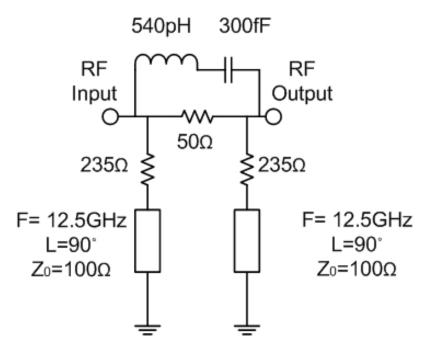
Figure 53: The schematic of designed conventional type gain-equalizer
