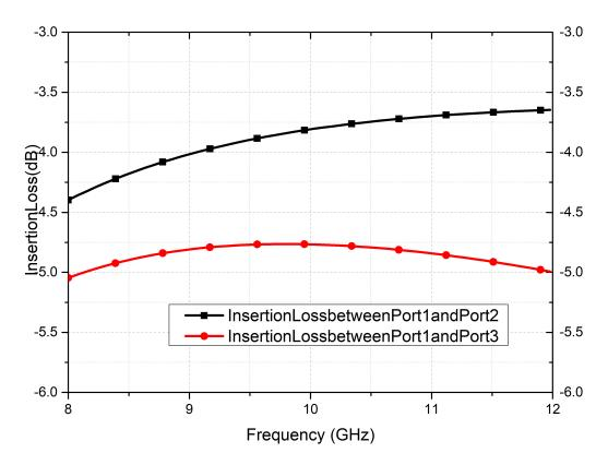
Figure 26: Simulation result of the insertion-loss between each output and input
