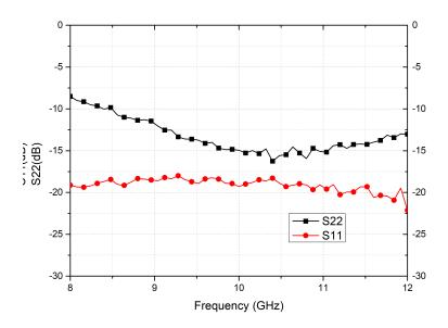
Figure 66: S11 and S22 measurement results of designed second active gainequalizer
