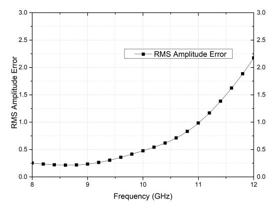
Figure 44: Simulation result of the RMS amplitude error of the designed phase shifter
