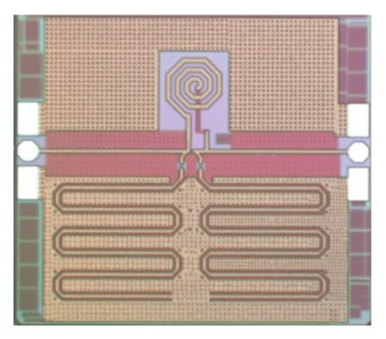
Figure 54: The micrograph of designed conventional type gain-equalizer
