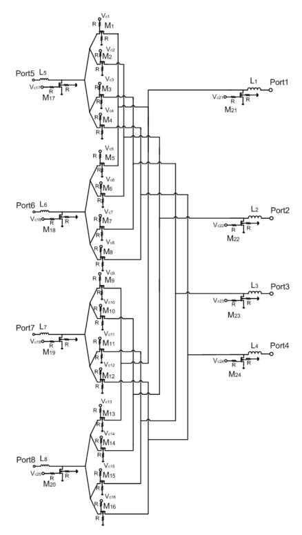
Figure 36: Schematic of the 4P4T
