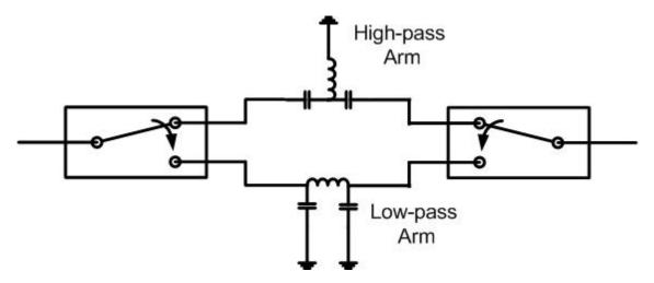
Figure 18: Switched-filter topology with tee networks
