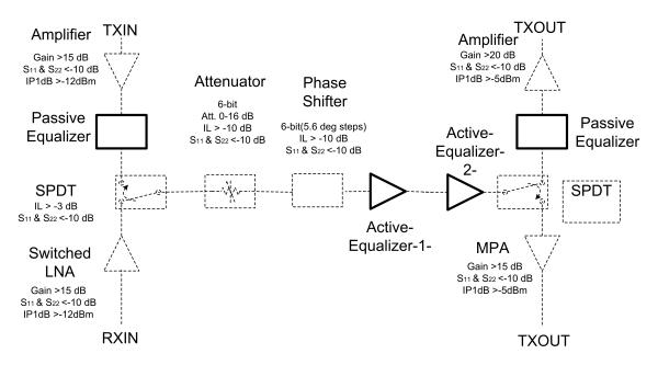
Figure 47: SiGe X-band all-RF T/R module block diagram and component specifications
