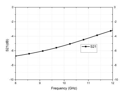
Figure 62: S21 measurement results of designed compact type gain-equalizer for TX chain
