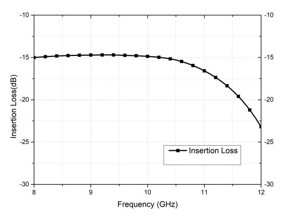
Figure 42: Simulation result of the insertion-loss of the designed phase shifter
