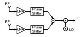
Figure 8: RF phase shifting Phased array architectures
