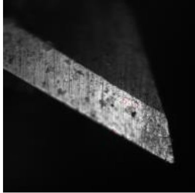
Figure 3.1 - Nanofocus image from a flute of a 2mm micro end mill
