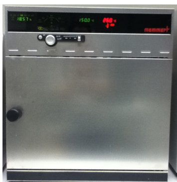
Figure 3.2: Oven used for hydrothermal treatment.
