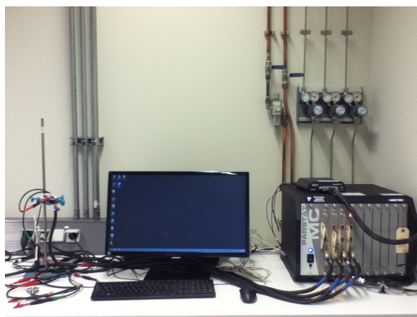
Figure 3.11: Battery test station for discharge and charge measurement.
