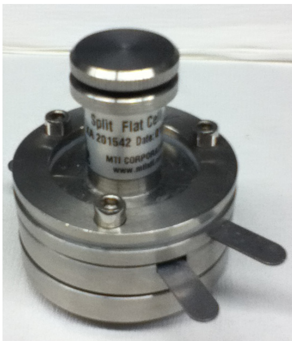
Figure 3.9: Stainless steel three-electrode split test cell.
