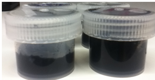
Figure 3.6: Slurry prepared by mixing the conducting additive of carbon black, PVDF binder in a mass ratio of 85:10:5 in a NMP solvent.
