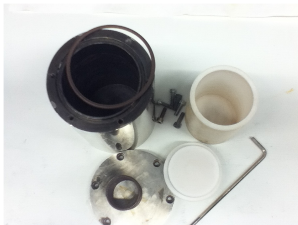
Figure 3.1: Image of the autoclave and Teflon beaker used for hydrothermal treatment.
