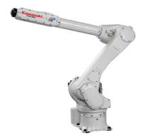
FIGURE 3.2: Six axis articulated robot [96]
