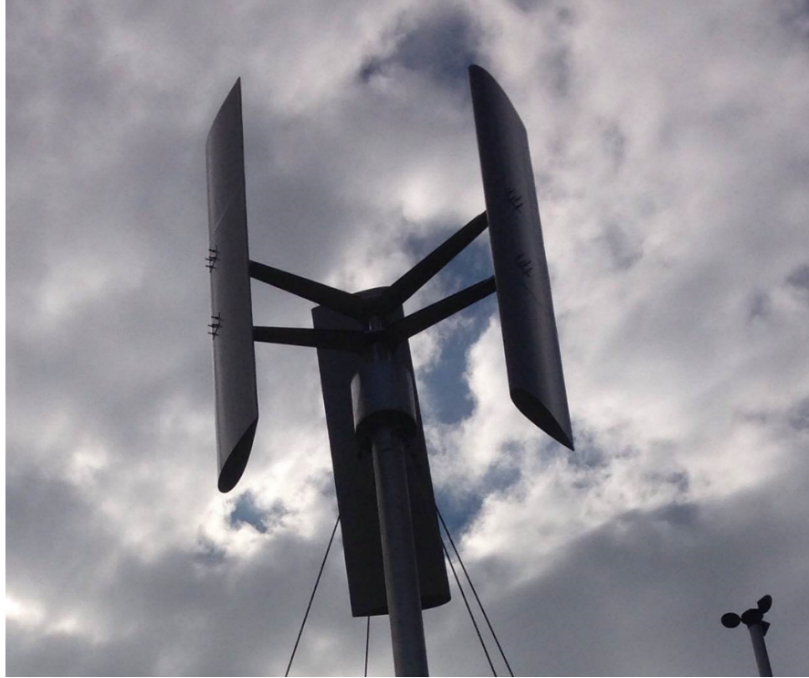
Figure 3.7: Experimental VAWT with the same dimensions used in the CFD model.
