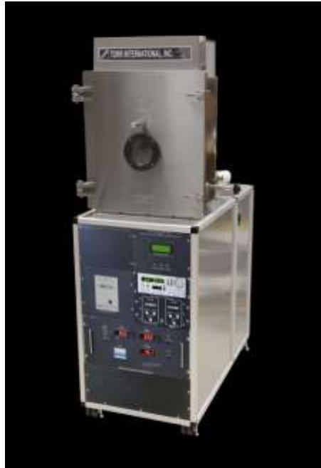
Figure 2.2. Torr e-beam evaporator used for alumina and iron layer coating
