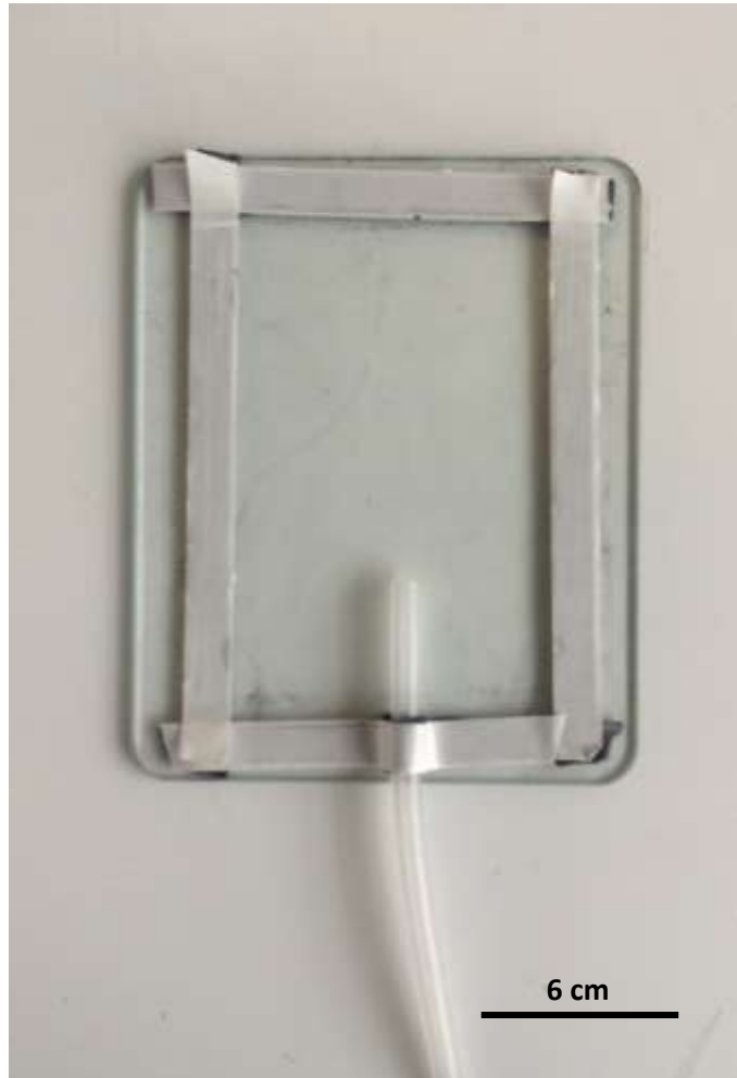
Figure 2.13. Glass plate with silicon tapes and pipe
