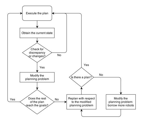
Figure 7.1: Flowchart of a local execution and monitoring algorithm
