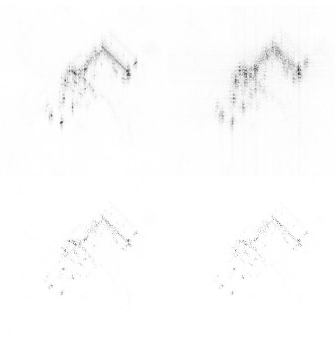
Fig. 3. a. Reference Backhoe image with 1-D phase error (upper-left), b. Zero-filled in Fourier domain reconstruction image (upper-right), c. Image reconstructed with autofocusing ADMM \ell_1 (lower-left), d. Image reconstructed with autofocusing ADMM \ell_{0.1} (lower-right)
