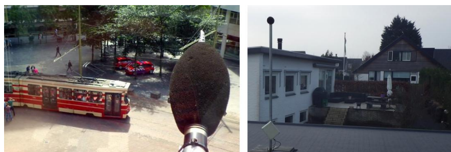
FIGURE 1.2: Microphones transmitting data in real time to Sensornet's database. Image retrieved from [2]
