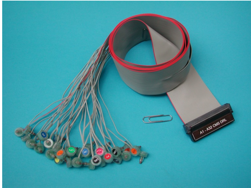
Figure 2.2: The BioSemi pin-type active electrode has a sintered Ag-AgCl electrode tip, providing very low noise, low offset voltages and very stable DC performance and completely resistant to long term water enabling easy cleaning and disinfecting. [3]
