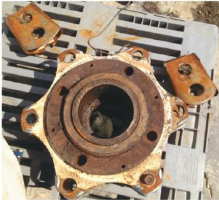
Figure 11. After 600 working hour, with hard metal welding
