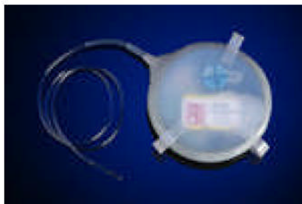
Figure 2.3 – A PA-D70 implant (Data Sciences International, Tilburg, Netherlands) used to measure maternal blood pressure and heart rate in pregnant sheep.
