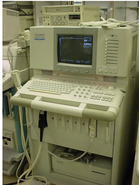
Figure 2.2 - Acuson 128 XP10 ultrasound machine (Siemens, Bracknell, United Kingdom) used to scan pregnant sheep and guinea pigs.
