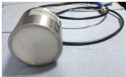
Figure 4-7 An image of the continuous wave ultrasound transducer PA 304 with a centre frequency of 0.66 MHz.
