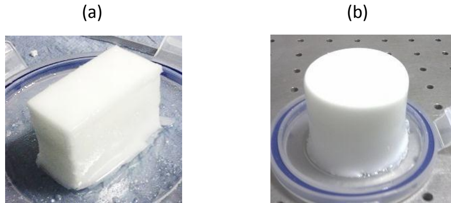
Figure 4-14 Samples of PVA gel phantoms of different shapes: (a) cuboid and (b) cylinder, which can be easily built by using appropriate moulds.
