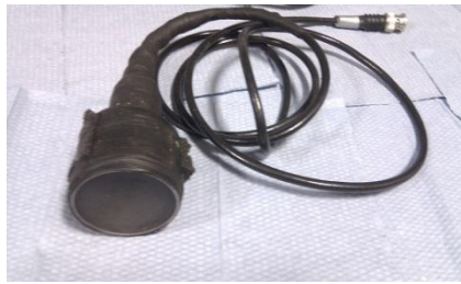
Figure 4-8 An image of the pulsed-wave ultrasound transducer of 1 MHz centre frequency.
