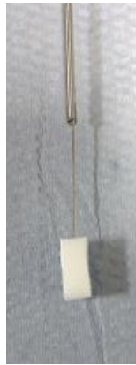
Figure 6-2 An image of the local scatterer, which has the \mu_s' of 20 \text{ cm}^{-1} and the \mu_a of 0.0235 \text{ cm}^{-1} . The local scatterer is held by a thin metallic rod, whose dimension is shown in Figure 5-5 (b).
