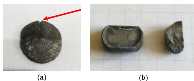
Figure 18. Titanium samples sintered by AC and tested by (a) compression with the red arrow identifying a fracture and (b) indirect tensile testing. The sample in (a) has a relative density of 71% and the samples in (b) have relative densities >80% (left) and <80% (right) with corresponding ductile and brittle behaviour, respectively.
