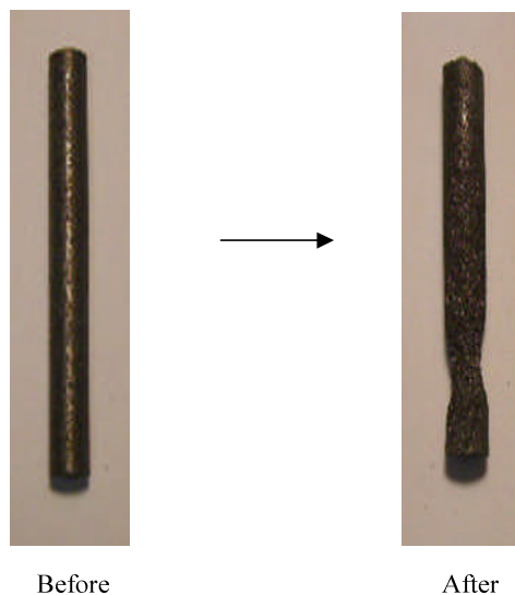
Figure 6-2: The pictures illustrate the 3 mm graphite WE before and after a flame experiment lasting 5 minutes. Although the aim of the Pt CE was to shield the sides of the WE from the flame, it is clearly visible that the flame erodes not only the tip but also the sides of the electrode.
