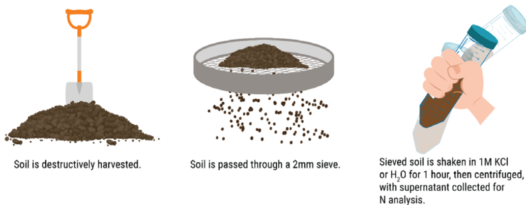
Figure 1-3. A simplified example of a soil extraction method. In the final step, salt extractant concentrations can vary, as can the type (KCl and K 2 SO 4 are both commonly used).
