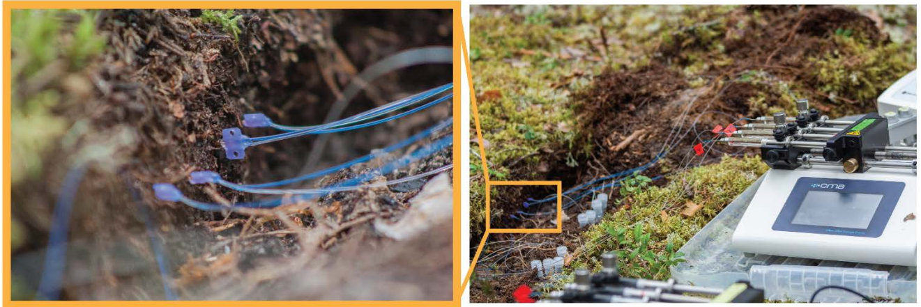
Figure 1-4. A microdialysis system being deployed in situ within the O horizon of a heath forest soil, near Umeå, Sweden.
