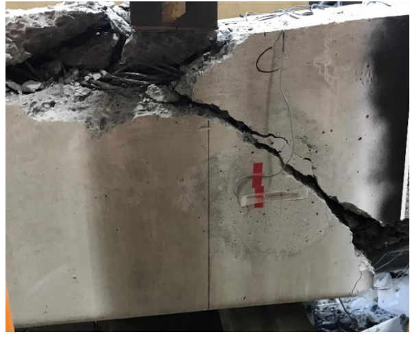
Point E. 760kN catastrophic failure, failure in compression zone and shear failure.
