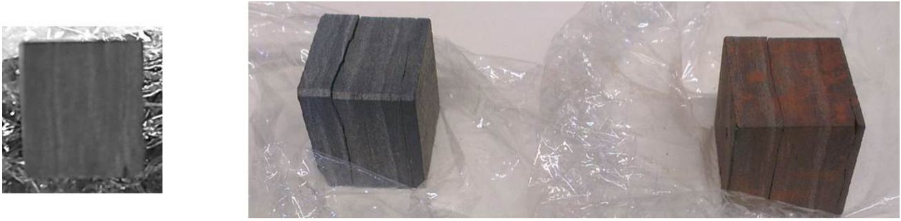
Figure 43: Precipice 1207.6 m core block photos, left before reaction, centre post reaction with CO 2 -brine (block A1), right post reaction with SO 2 -CO 2 -brine (block A2), note red-brown colouration.
