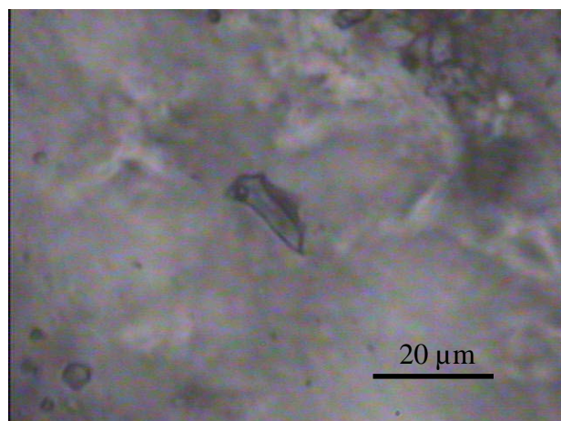
Aqueous, two phase fluid inclusion and smaller liquid-only inclusions in quartz overgrowth
