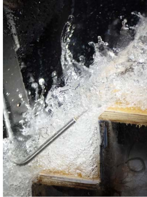
(A) Laboratory experiment - Q = 0.084 \text{ m}^3/\text{s} , Re = 3.4 \times 10^5 , h = 0.10 \text{ m} , \theta = 45^\circ
