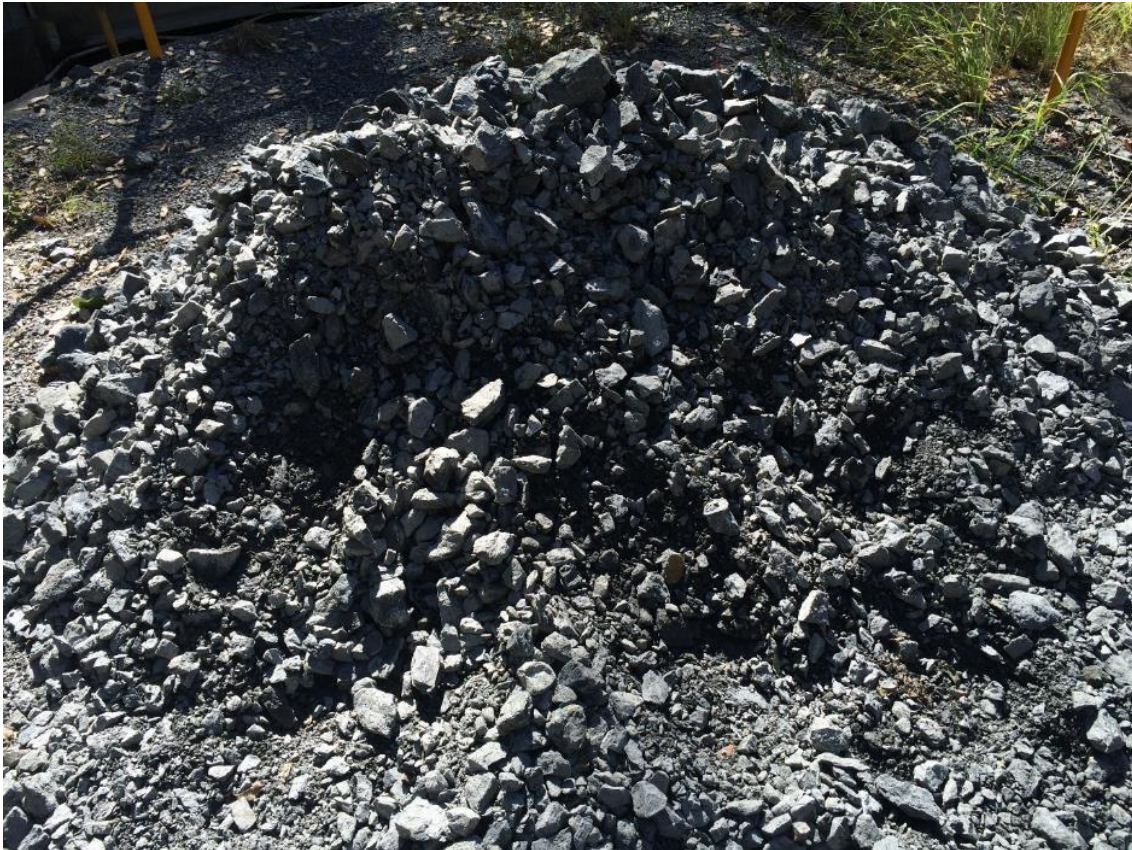
Figure 1 Crusher run (-75 mm MC-CR) from Mt Coo-Tha Quarry, Brisbane
