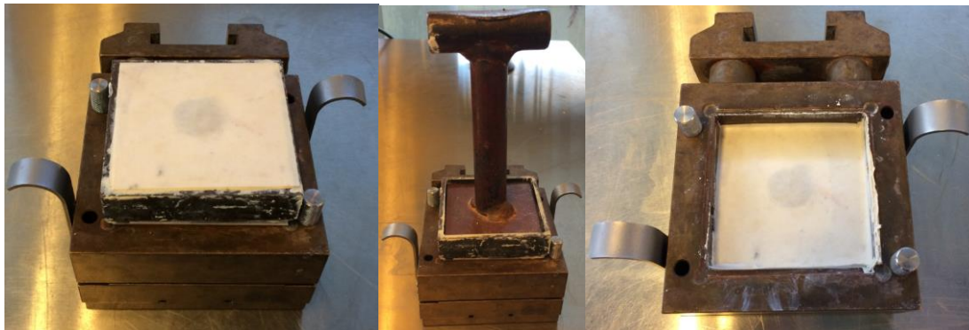
Figure 3 Kaolin with sand column in shear box
