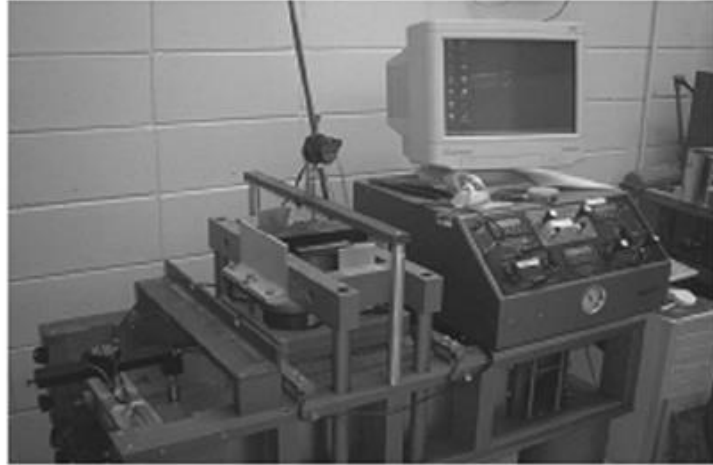
Figure 2.4 Large-scale direct shear machine (Abu-Farsakh et al. 2007)
