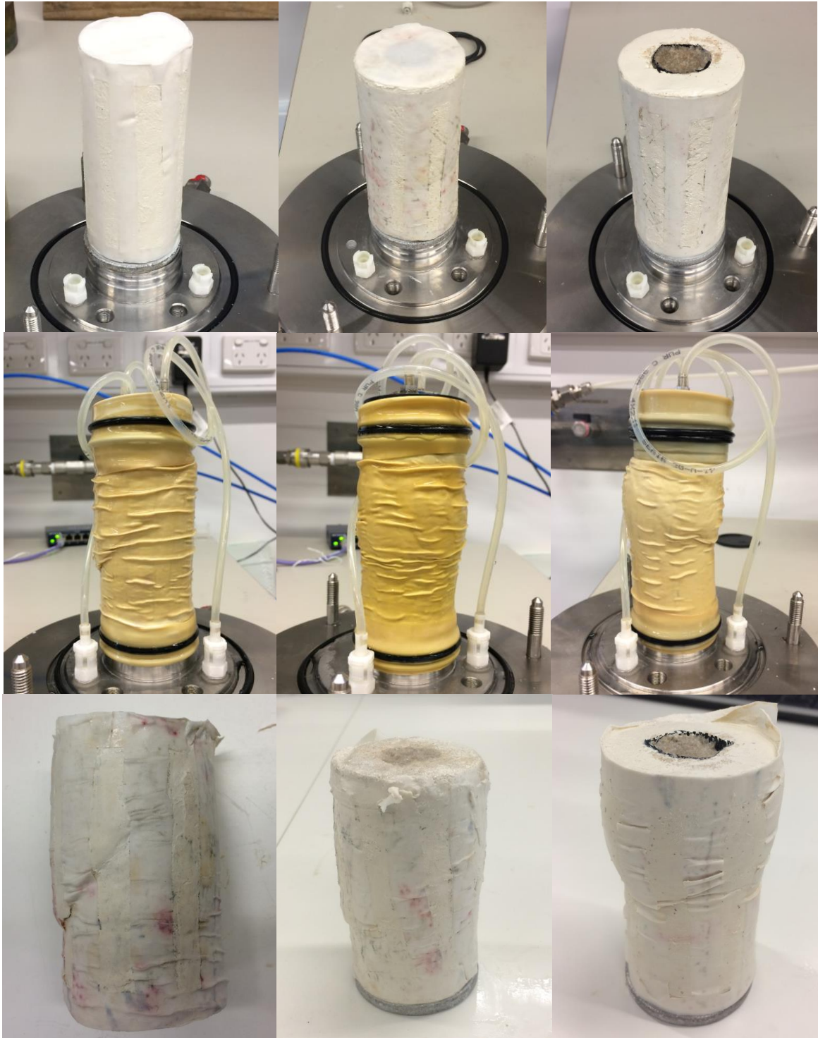
Figure 9 Photos of Kaolin, Kaolin with OSC and Kaolin with GESC specimens in CU triaxial tests before and after failure
