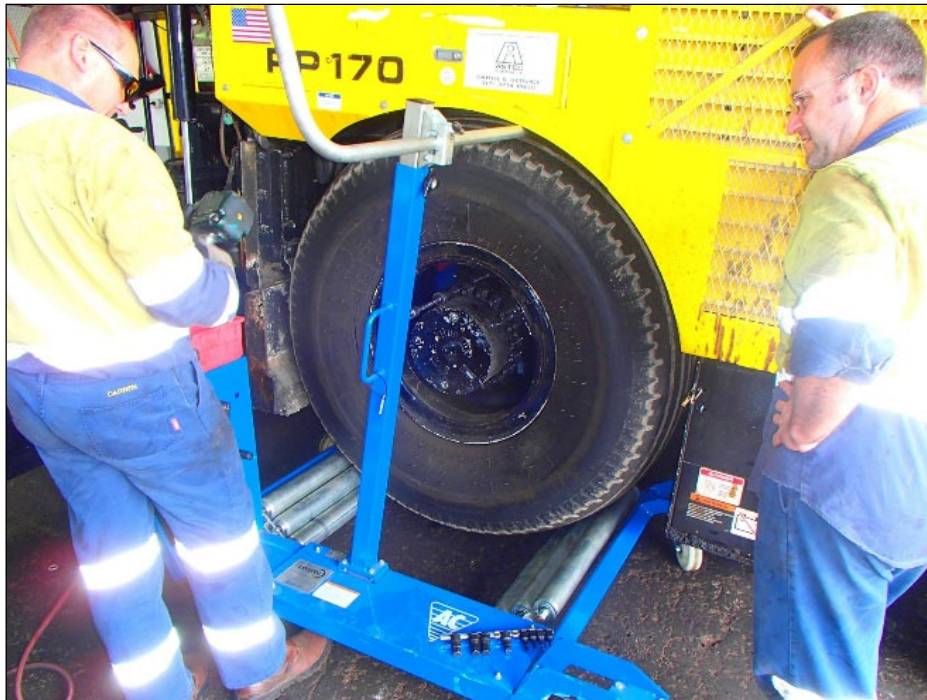
Figure 3.17: The use of a wheel dolly to eliminate the forklift use
