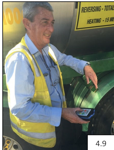
Figures 4.9 – 4.10: Simulated trial of remote control for lever operation for bitumen transfer; Remote-operated lever
