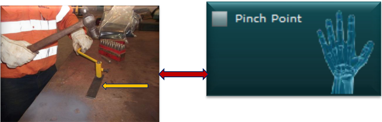
Figure 6.3: A design improvement to isolate hands and fingers from hammer blows
