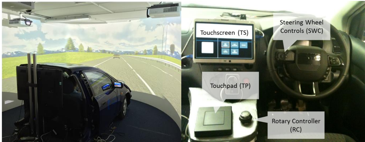
Figure 1: Experimental set-up in the UK, showing medium-fidelity driving simulator and device locations
