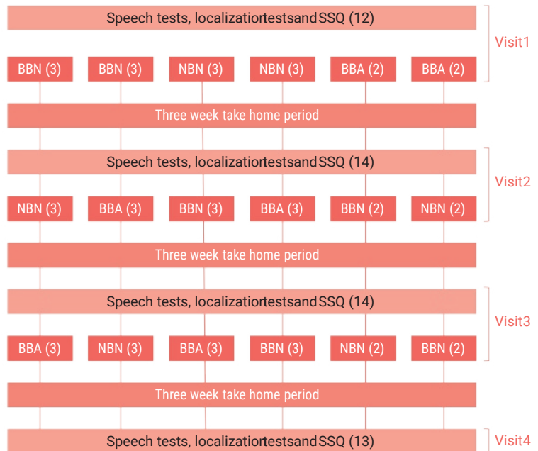
Figure 2 Subjects were randomly distributed over the six arms of the cross-over study. The numbers between parentheses are the number of subjects. BBN denotes broadband balancing of NALNL-2 fitting formula, NBN denotes narrowband balancing of NALNL-2 fitting formula, and BBA denotes broadband balancing of Audiogram+ fitting rule.
