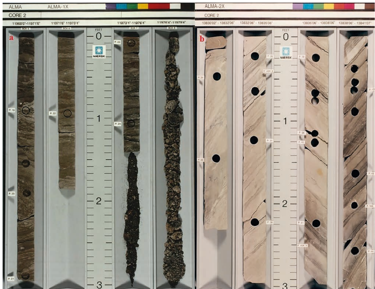
Fig. 5. Overview of representative core parts. Left: Alma-1X. Right: Alma-2X. The core quality of Alma-1X is considered moderate to good while the general quality of Alma-2X is considered to vary from good to very good due to the larger core diameter and more coherent cores. Alma-2X is not vertical, which results in the steep apparent dip of the strata (Fig. 4). Photographs by Maersk Oil. Scale in feet. Core parts shown are for Alma-1X: 11900'00''–11979'04'' (core 2), and for Alma-2X: 13830'02''–13841'07'' (core 2).
