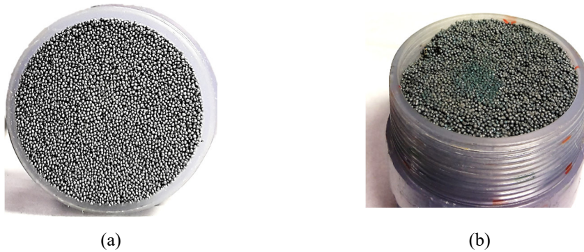
Figure 4-19. The AMR with five layers of packed spheres (a) before and (b) after testing in the Test machine .
