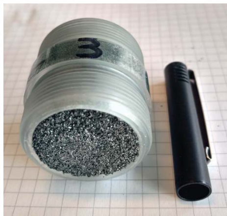
Fig. 1 : Photo of an epoxy bonded regenerator, pen top for scale.
