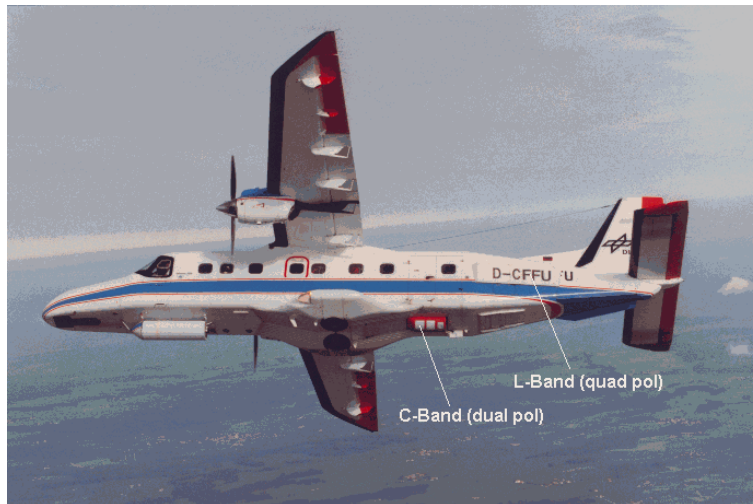
Figure 4-3. Photograph of the Dornier DO-228 aircraft used for the E-SAR campaign over Horns Rev on 12 October 2003. Positions of the C-band and L-band SAR sensors are indicated (from http://www.dlr.de/hr/institut/abteilungen/sar-technologie/fg/flugzeug-sar/ )
