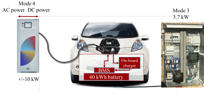
Fig. 2. Physical setup - Nissan LEAF with different charging options
