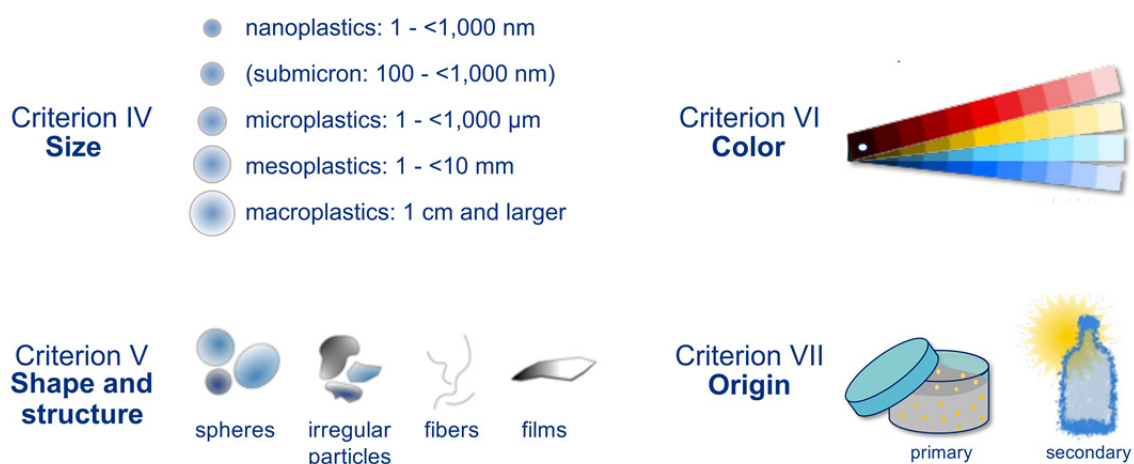
Figure 1. A definition and categorization framework for plastics as proposed by Hartmann et al. (2018 - Paper VIII). Figure modified from Hartmann et al. (2018 - Paper VIII).
