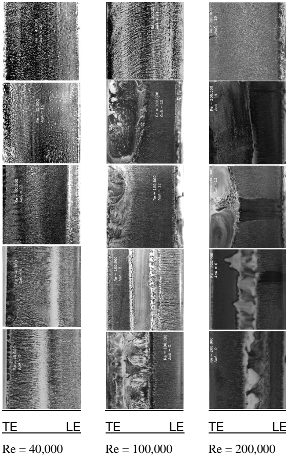
Figure 5: Oil-flow visualisations at various Reynolds numbers and angles of attack 20°, 15°, 12°, 6°, and 0° from top to bottom.
