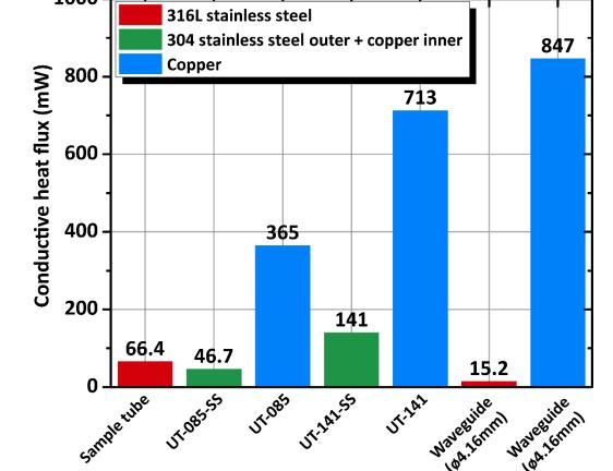
Thermal heat coupled by a coaxial cable can be significant (particular via the inner conductor). A compromise between electrical loss and thermal loading can be achieved using a
