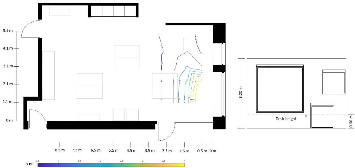
Figure 6.12: Daylight factor level [%] at 0.6m above floor level in room 1.2.06 (left). Façade window layout of the classroom as seen from outside the room (right). Glazing-to-floor-area-ratio = 26%
