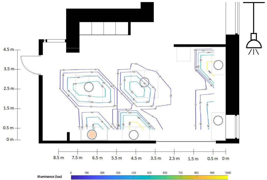
Figure 6.8: Illuminance levels [lux] at 0.6m above floor level in room 1.2.06 under New Scenario C - Focused Pendants (100% output ) for electric lighting only.
