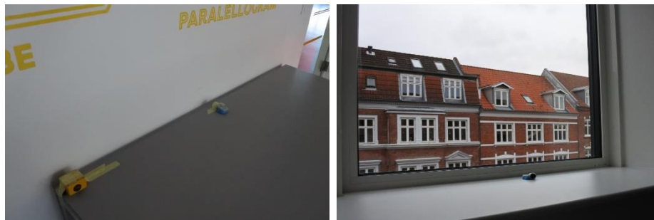
Figure 3.19: On the left, temperature (yellow Tinytag) and illuminance meter (HOBO) at working area at the back of room 1.2.10. On the right, lux meter on windowsill in room 1.2.06.
