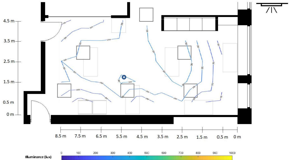
Figure 6.4: Illuminance levels [lux] at 0.6m above floor level in room 1.2.10 under New Scenario A - Ambient Ceiling Lighting (70% output) for electric lighting only.
