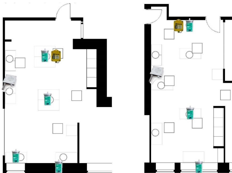
Figure 3.20: Location of CO 2 , temperature and illuminance meters in room 1.2.06 (left) and 1.2.10 (right).
