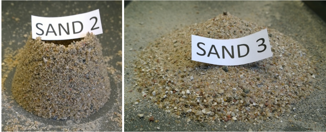
Fig. 7 – Sand tested with the cone method. Left: Moisture content u=3.0\% , where menisci formation in the interparticle water generates cohesive forces – “interstitial liquid bridges” – between the sand particles and retains the shape despite removal of the mold. Right: Moisture content u=0.3\% , where the moisture content is below the SSD state. Due to absence of sufficiently strong interparticle forces, in this case notably absence of interparticle water, the sample slumps completely when the mold is removed.
