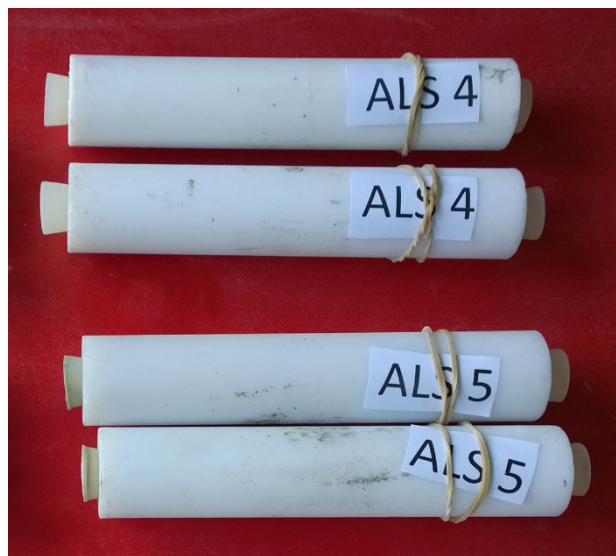
Fig. 5 – PTFE tubes with an internal diameter of Ø14 mm and length 150 mm. The tubes were filled with the particulate sample and closed with rubber bungs in both ends.
