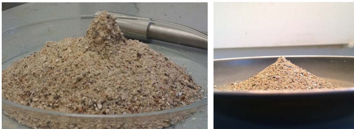
Fig. 2 – Sand tested according to ASTM C128 [7] and EN 1097 [3]. Photos are taken right after removal of the conical mold. Left: The moisture state is at a level where the complete particle cone has just achieved slump, i.e. no contours of the original cone shape exists. This is the SSD state according to ASTM C128. Right: The particle cone has slumped into the angular slopes required by the EN 1097 definition of the SSD state. Perhaps a tiny, slightly concave tip is still visible, indicating that the moisture state is just above the SSD state according to EN 1097.
