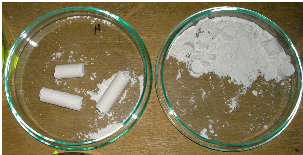
Fig. 9 – Frozen alusilica samples after demolding. Left: Moisture content u=16.6\% , where the sample has considerable strength with notable particle cohesion. Right: Moisture content u=12.4\% , where the sample disintegrates into powder during demolding – the small pieces seen have no relevant cohesion and disintegrate at the slightest touch.
