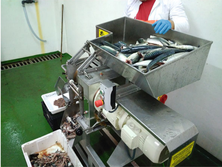
Fig. 17.4 iDVP1 fish fractions separator
