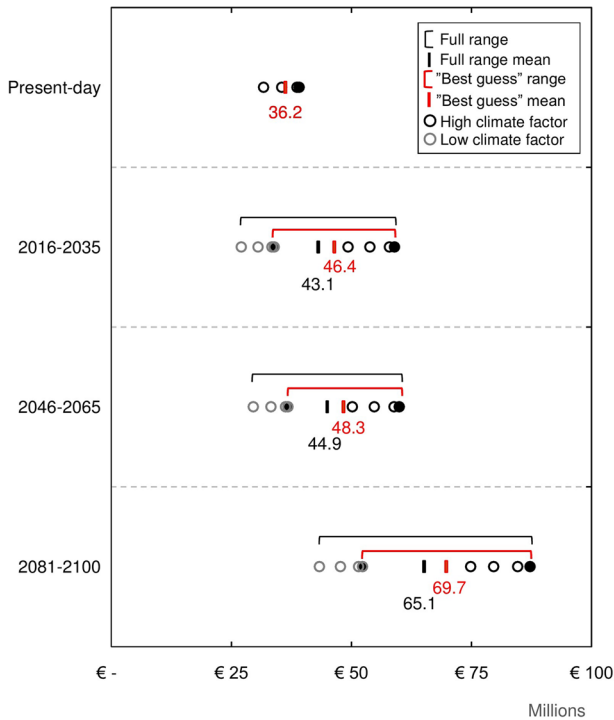
Fig. 6 Variation in damage costs to buildings during flooding from extreme precipitation with a 100-year return period (RP100) using different assumptions about the time horizon of climate change scenarios, climate model projections, building property values, and infiltration data. Damage costs are estimated for four periods: present-day, 2016–2035, 2046–2065, and 2081–2100. The individual circles represent different assumptions regarding climate scenario and models, building property values, and infiltration. Gray/black circles represent a low/high degree of climate change and refer to the lowest/highest values in precipitation intensity in the “RCP4.5 and RCP8.5” column in Table S1 in the supplementary material, which represent the 10th and 90th percentiles of the ten GCMs. The solid gray and black circles highlight the “best-guess” estimates for building damage costs, where location-specific building values and location-specific infiltration are used. The “best-guess” range is shown as the variation between the solid gray and black circles, while the full range represents the total variation of all estimates
