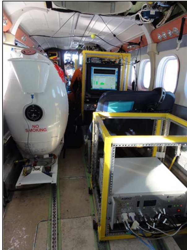
Figure 4: Picture taken from the back of the Twin Otter. ASIRAS instrument is in the aft rack and control computers in the other rack. The Honeywell INS is mounted under the seat.
