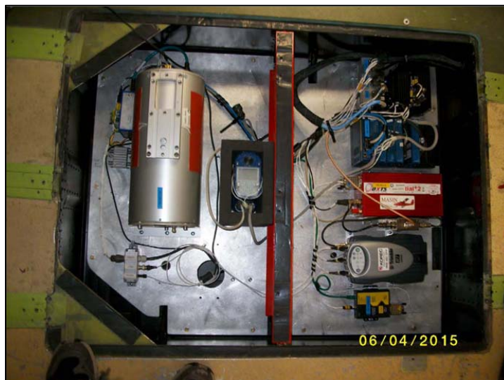
Figure 2: Instrument installation in the camera bay below the floor in the Twin Otter. ALS (left), OxTS INS (middle right) and Trimble GPS receiver (lower right). Note ALS and OxTS INS axis are mounted along the aircraft center line.
