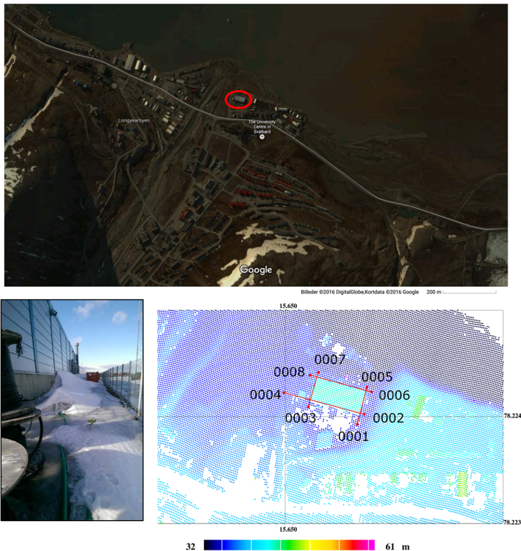
Figure 4 Calibration building in Longyearbyen. Location (upper plot), measurement of the building (lower left) and ALS DEM of the building together with markings of the measurement points (lower right).
