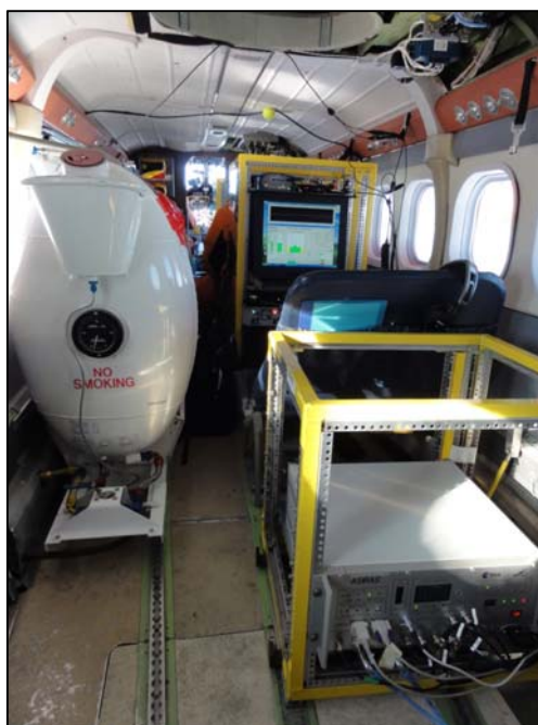
Figure 3 Picture taken from the back of the Twin Otter. ASIRAS instrument is in the aft rack and control computers in the other racks. The Honeywell INS was mounted on the floor under the seat.
