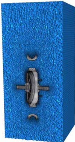
Figure 8. The mesh for external flow simulation.
