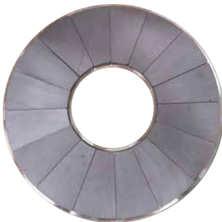
Figure 6.29: The ferrite magnet poles and rotor yoke assembly of the SAT PMLDC motor.
