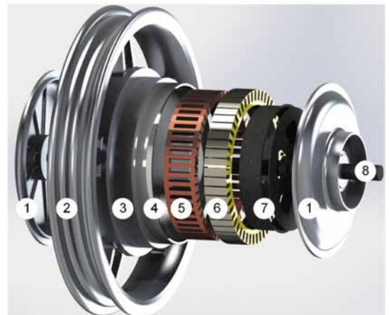
Figure 1. Exploded view of the motor (1. Endplate, 2. Rim, 3. Rotor core, 4. Magnet, 5. Winding, 6. Stator core, 7. Spider and 8. Non rotating shaft).
