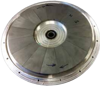
Figure 6.31: The end cover of the ferrite magnet SAT PMBLDC motor with the rotor attached.
