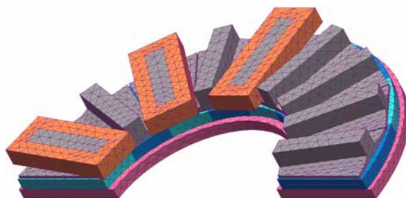
Figure 4.7: The FE model of SAT PMBLDC motor used in the design synthesis of in-wheel motor.
