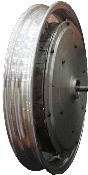
Figure 6.16: The fabricated prototype of bonded RE magnet SAT PMBLDC motor.
