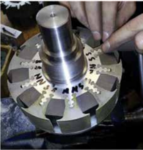
Figure 2.8: Rotor of a spoke type IPM motor using ferrite magnet [40]. © 2016 IEEE.
