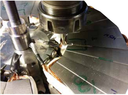
Figure 6.27: Creating slots for hall sensors on the completed stator assembly of the ferrite magnet SAT PMLDC motor.
