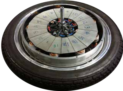
Figure 6.33: The ferrite magnet SAT PMBLDC motor assembly right after the stator is inserted into the spacer with an end cover assembly.
