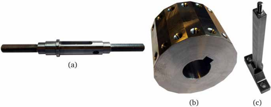
Figure 6.24: The shaft, the hub, and a tooth holder of the ferrite magnet SAT PMLDC motor.
