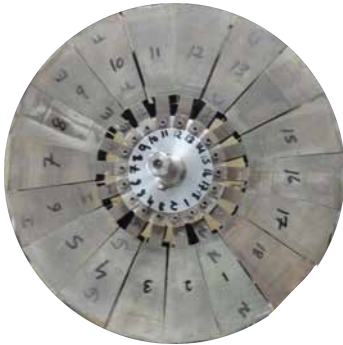
Figure 6.12: The stator assembly of the bonded RE magnet SAT PMBLDC motor without winding.
