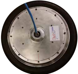
Figure 6.34: The fabricated prototype of ferrite magnet SAT PMBLDC in-wheel motor.
