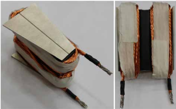
Figure 6.23: The stator tooth of the ferrite magnet SAT PMLDC motor wound with 30 turns of stranded copper wire.
