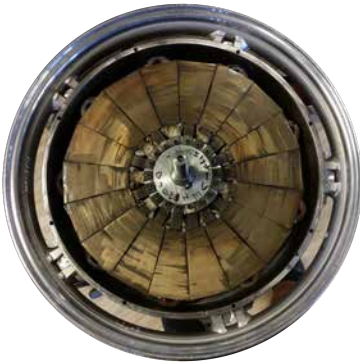
Figure 6.14: The bonded RE magnet SAT PMBLDC motor assembly right after the stator is inserted into the spacer with an end cover assembly.
