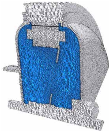
Figure 14. Meshed model for internal flow with polyhedral mesh of 3.5 mm base size.
