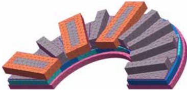
Fig. 6. FE model of the SAT PMBLDC motor used in the design synthesis of the in-wheel motor.
