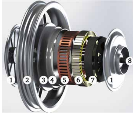
Figure 7.3: Exploded view of the radial flux sintered RE magnet motor of vehicle-1 (1. End plate, 2. rim, 3. rotor core, 4. magnet, 5. winding, 6. stator core, 7. spider and 8. non rotating shaft).
