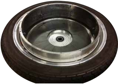
Figure 6.32: The rotor wheel and spacer assembly of the ferrite magnet SAT PMBLDC motor with attached end cover.
