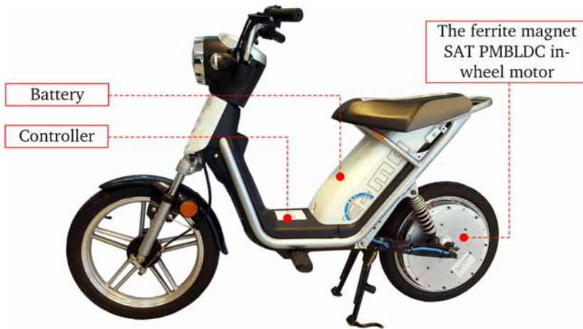
Figure 6.35: The ferrite magnet SAT PMBLDC motor installed in a two wheeler.
