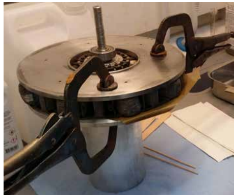
Figure 6.15: Applying resin to the aligned stator of the bonded RE magnet motor.
