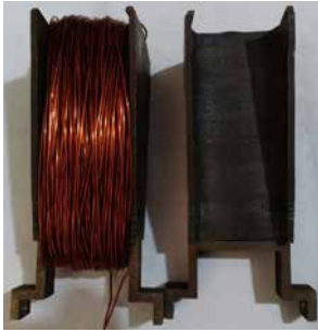
Figure 6.10: The segmented stator tooth with and without coil.
