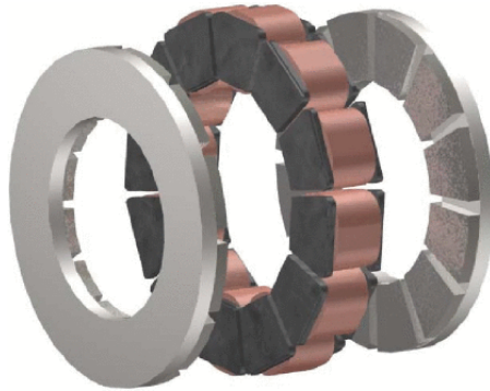
Figure 2.12: Segmented armature torus permanent magnet motor [64]. © 2007 IEEE.
