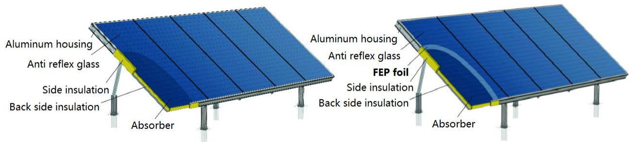
Fig. 3 Typical large flat plate collectors without/with FEP foils used in solar heating plants (Source: Arcon-sunmark A/S) [33].
