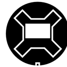
Fig. 5. Meandered slot loop on-body antenna type. The rectangular battery compartment is shown in white in the center [36].
